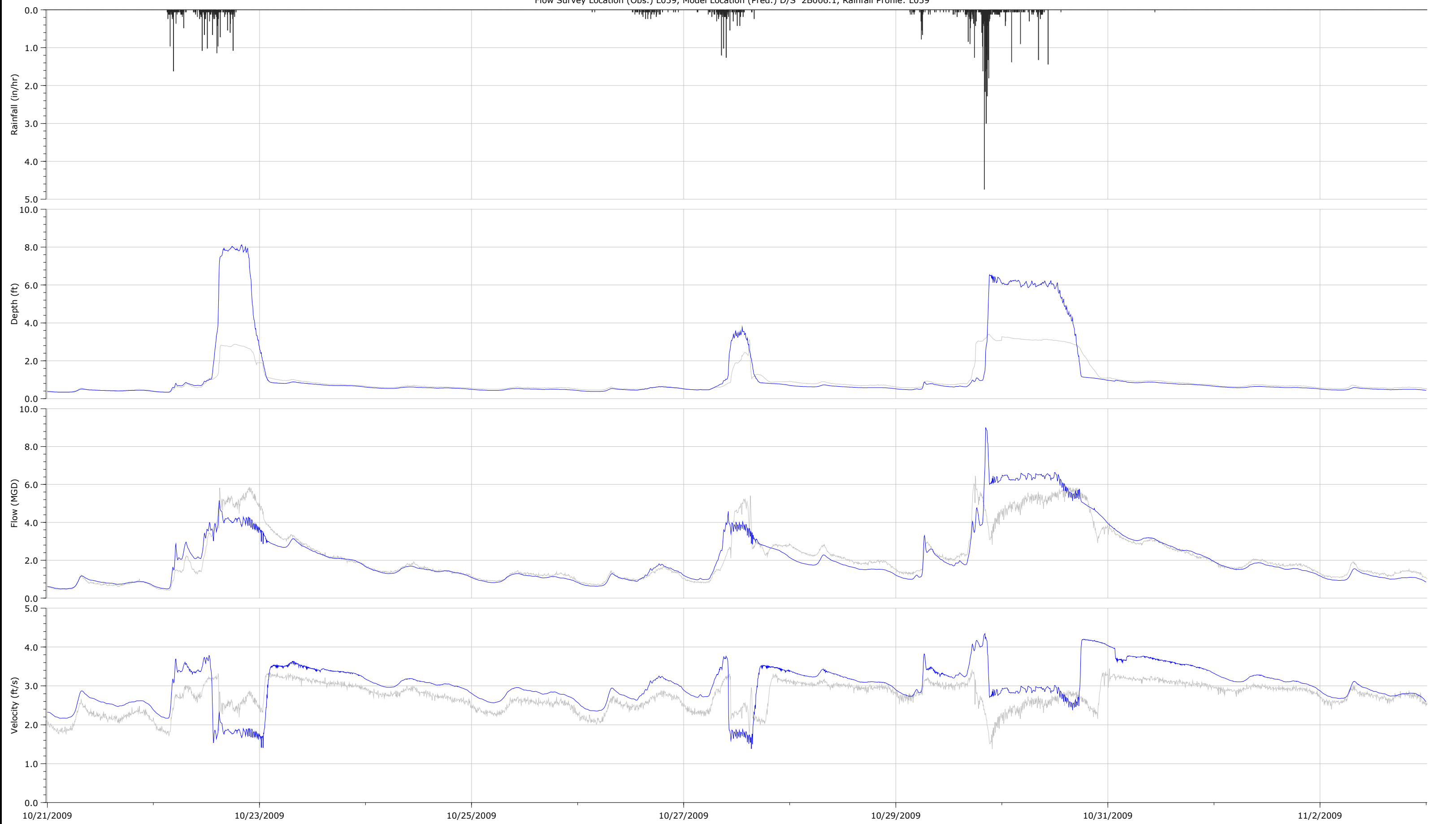
Flow Survey Location (Obs.) L059, Model Location (Pred.) D/S 2B006.1, Rainfall Profile: L059
