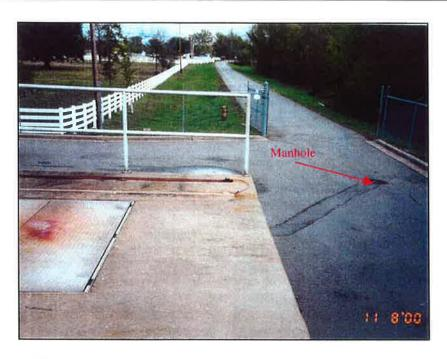
Figure 13. Manhole to be used for location of flow meter.
